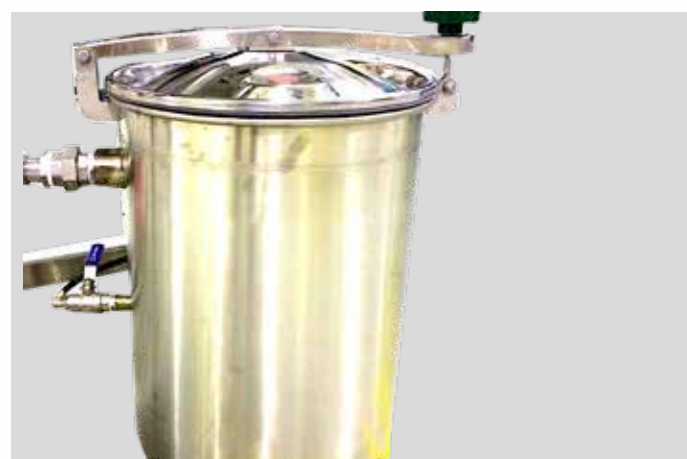
TANICA ACCUMULO SOLVENTE E DEPOSITO INCHIOSTRO SOLVENT STORAGE TANK AND INKDEPOSIT
