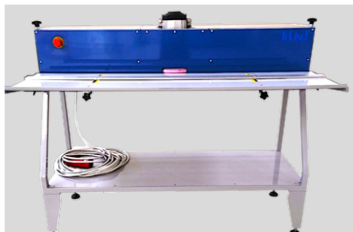
AFFILA RACLE VISTA FRONTALE SQUEEGEE'S SHARPENER FRONT VIEW
