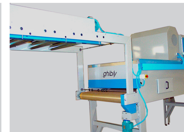
GHIBLY GAS CON USCITA PER GESTIONE NASTRI GHIBLY GAS WITH EXIT FOR NARROW FABRIC TAPE
