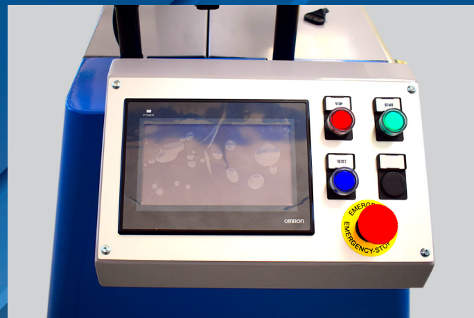
PANNELLO DI CONTROLLO PRINTING CONTROL PANEL
