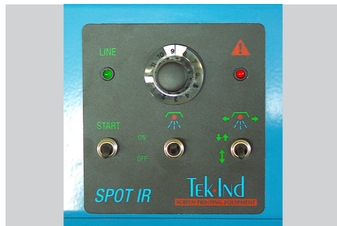
PANNELLO COMANDI SPOT SERIE IR CONTROL PANEL ON SPOT IR SERIES
